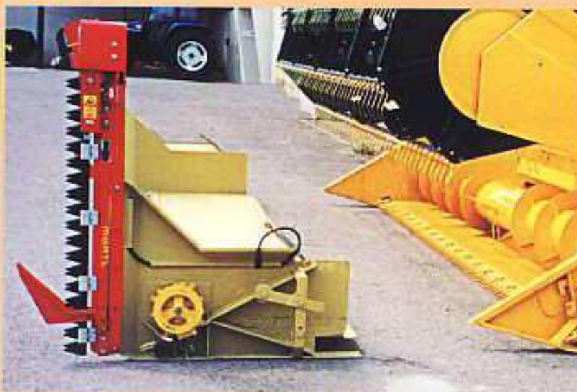
Header extension before fitting
